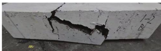
Fig. 6—Cracking pattern on bottom of beam specimen 1-2.
