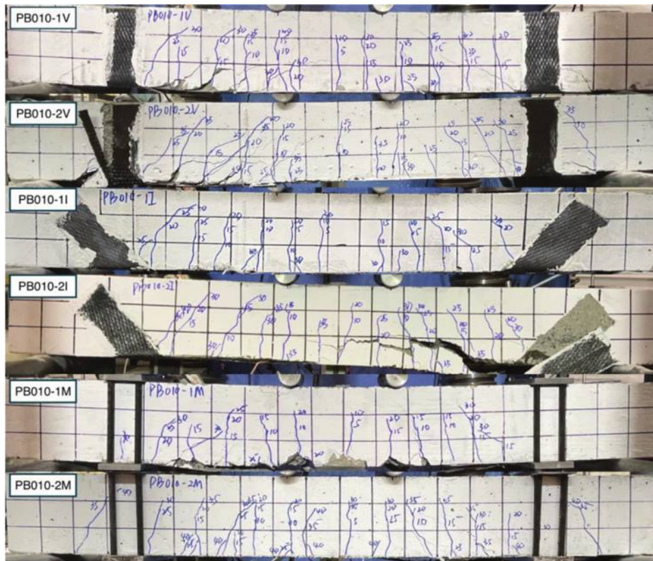
Fig. 10—Crack patterns of PB010 series.
