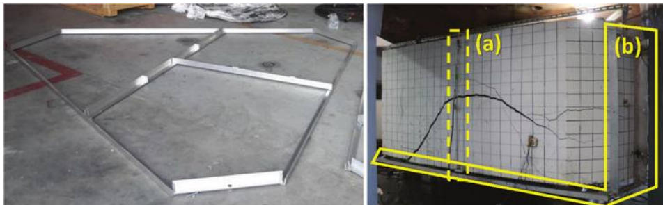
Fig. 5—(Left) underhung truss for bottom transducers; and (right) photograph of Specimen L3h showing: (a) transducer to measure side crack width; and (b) mounting of underhung truss.
