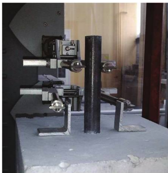
Fig. 4—Extensometer mounted at free end of plain steel bar during testing.
