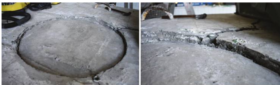
Fig. 12—Vertical settlement of top bearing area (Specimen L3a).
