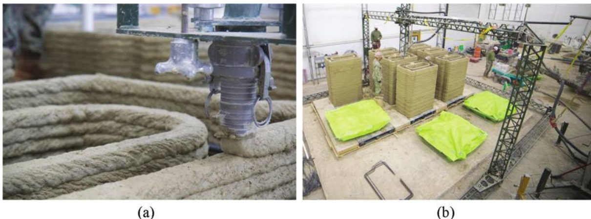
Fig. 1—AC process: (a) material extrusion; and (b) printing machine. (Note: U.S. Army Corps of Engineers images by J. Eastman.)
