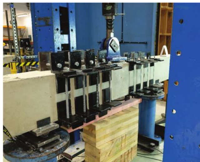
Fig. 15—Test setup for beams.
