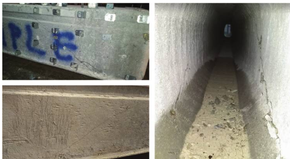
Fig. 10—Web-shear cracking in shear span F2-40-3.5b (left: exterior webs; and right: interior web).
