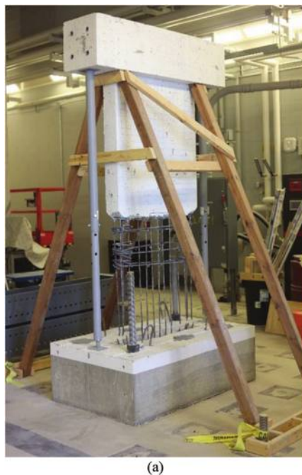
Fig. 4—Final stage of concrete removal: (a) SWS-R; and (b) SWN.
