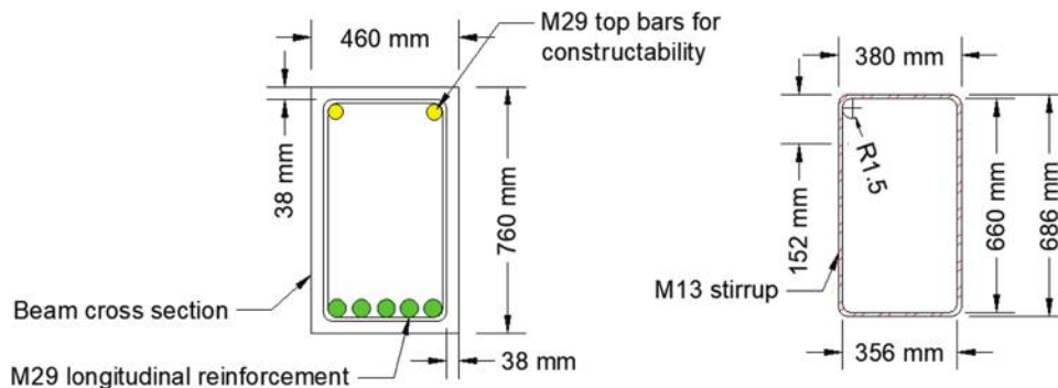
Fig. 3—Beam cross section and stirrup dimensions at midspan.
