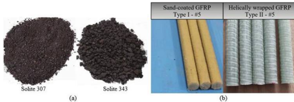
Fig. 1—(a) Lightweight aggregates; and (b) GFRP reinforcing bars.
