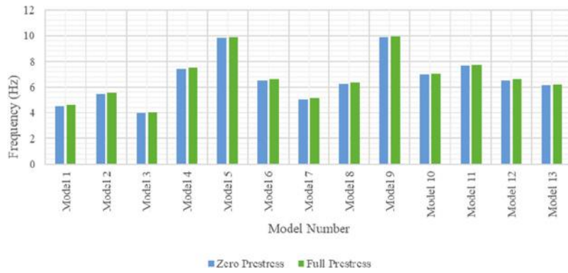
Fig. 14—Fundamental frequencies of concrete slabs with linear material behavior and applied load of 6 kN/m 2 .
