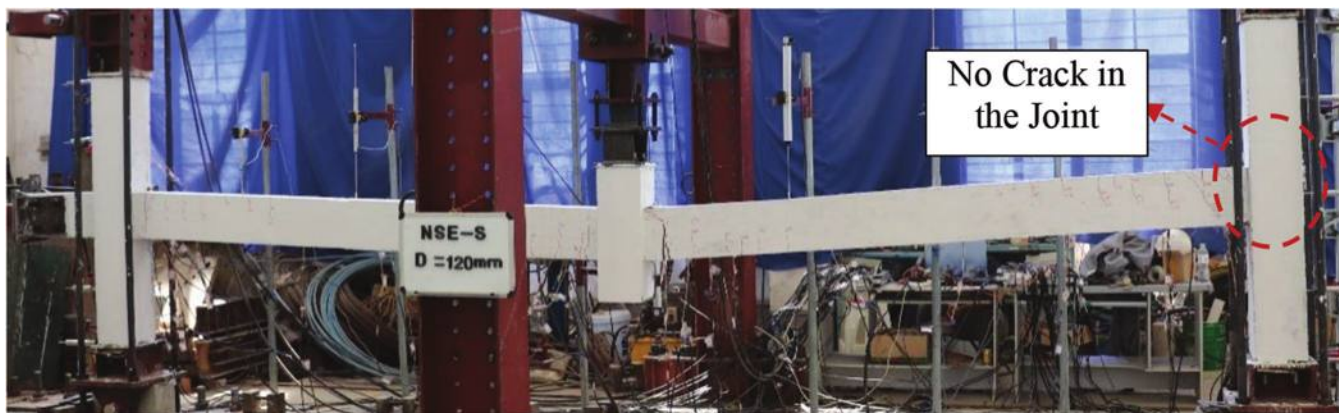
Fig. 15—Crack pattern of OP-S at displacement of 120 mm (4.7 in.).
