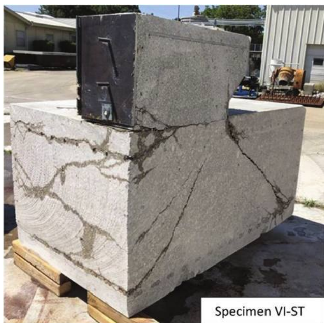
Fig. 15—Internal cracks formed across width of specimen VI-ST.
