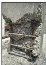
Buckled rebar at column base @ 6 % lateral drift
