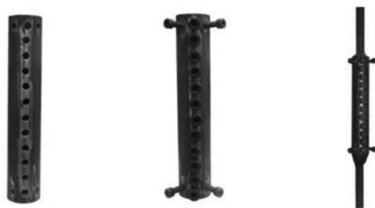
(b) Proposed coupler sleeve with bolting and rebar-interlinking arrangement
