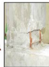
Ruptured rebar at column base @ 6 % lateral drift
