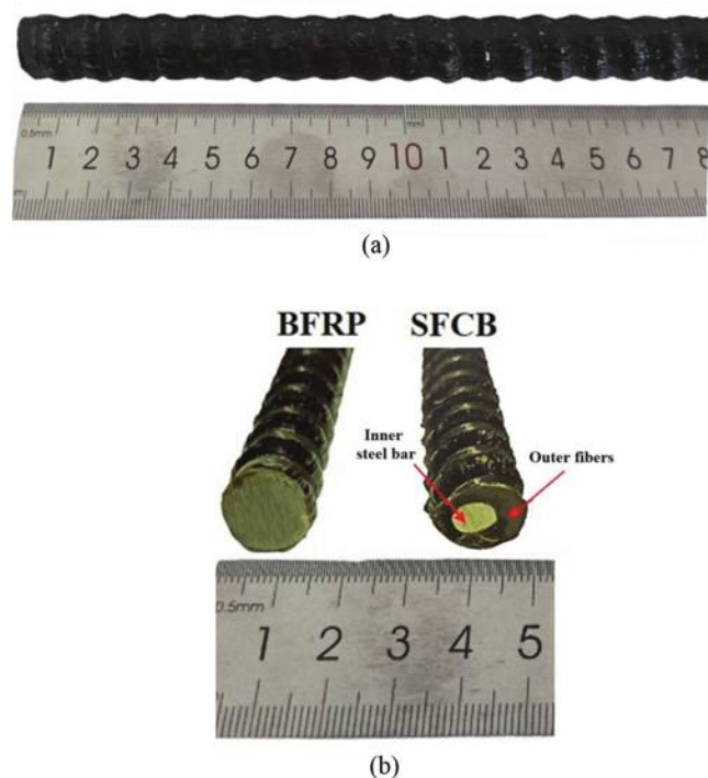
Fig. 1—Configuration of BFRP and SFCB reinforcing bars: (a) geometry of BFRP bars and SFCBs; and (b) cross sections.
