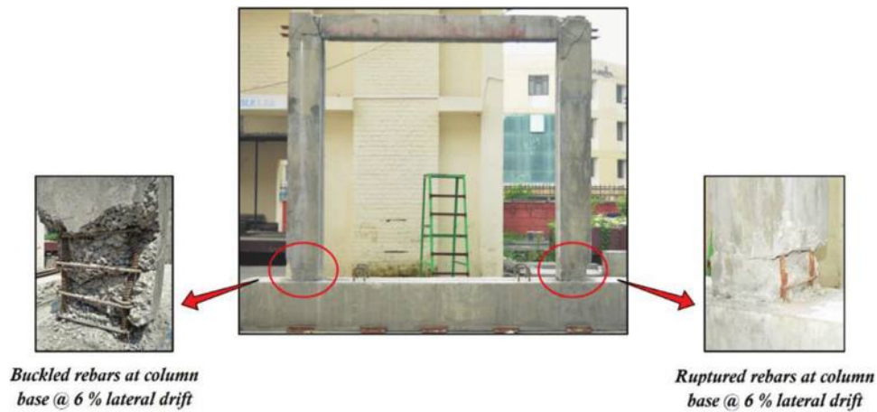
Fig. 11—Damaged model frame after preliminary test.
