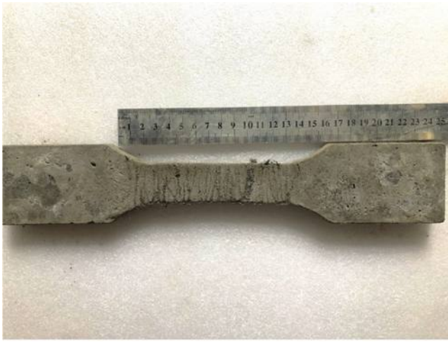
Fig. 8—ECC multiple tight microcracks of E-2.2 direct tension test specimen.
