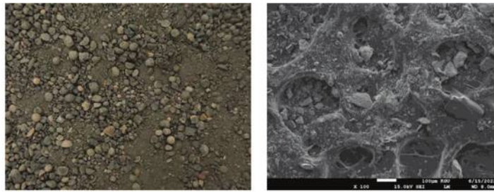
(a) Expanded clay granule for fine aggregate
