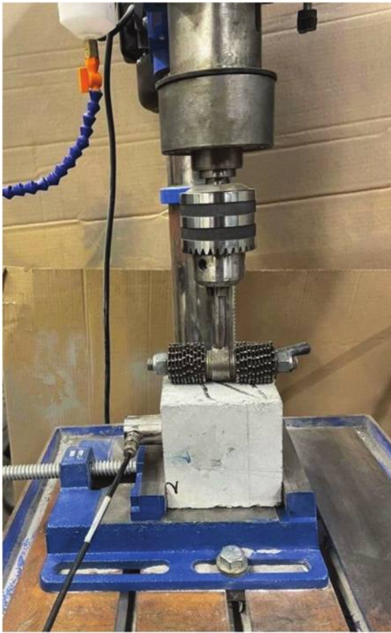
Fig. 1—AE and rotating-cutter abrasion test setup.
