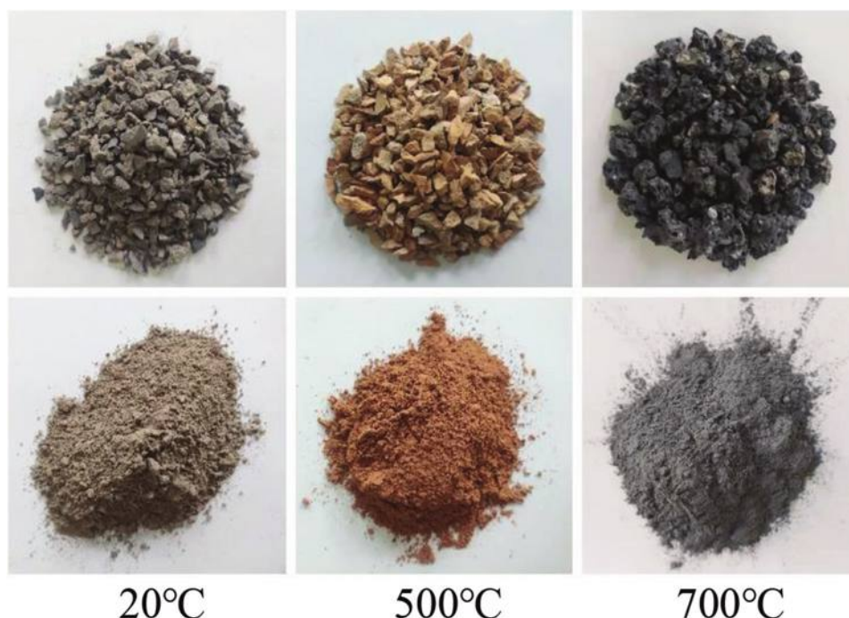
Fig. 3—Appearance of coal gangue calcined at different temperatures.
