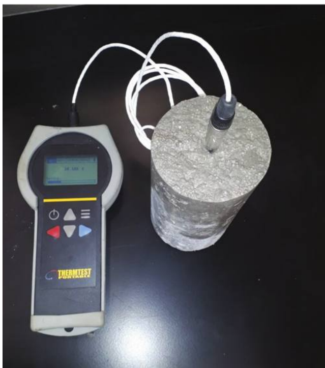
Fig. 5—Thermal conductivity measurement of ECCs.
