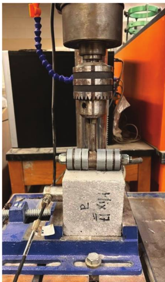
Fig. 2—Verification abrasion test setup using smooth roller.
