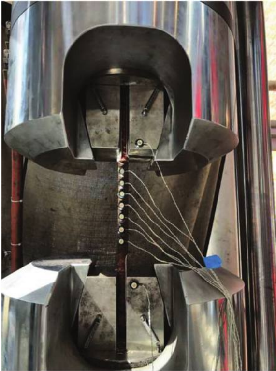
Fig. 6—Tension test setup on corroded reinforcing steel bar.
