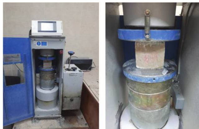
Fig. 7—Optical photos during measurement of compressive strength.
