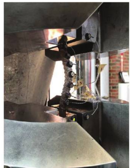
c) Buckled bar in compression
