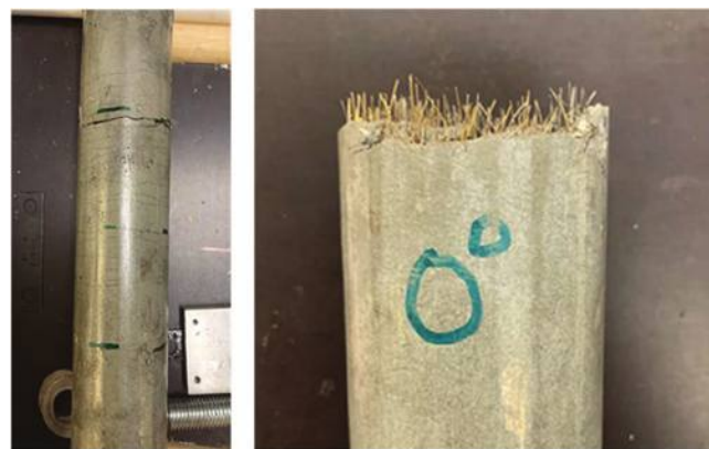
Fig. 8—Typical crack pattern and fiber orientation for 0-degree casting.
