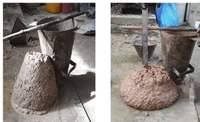
Fig. 8—Live photos during slump measuring.
