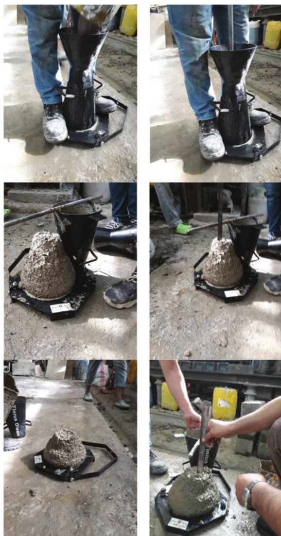
Fig. 4—Optical photos during slump measuring.
