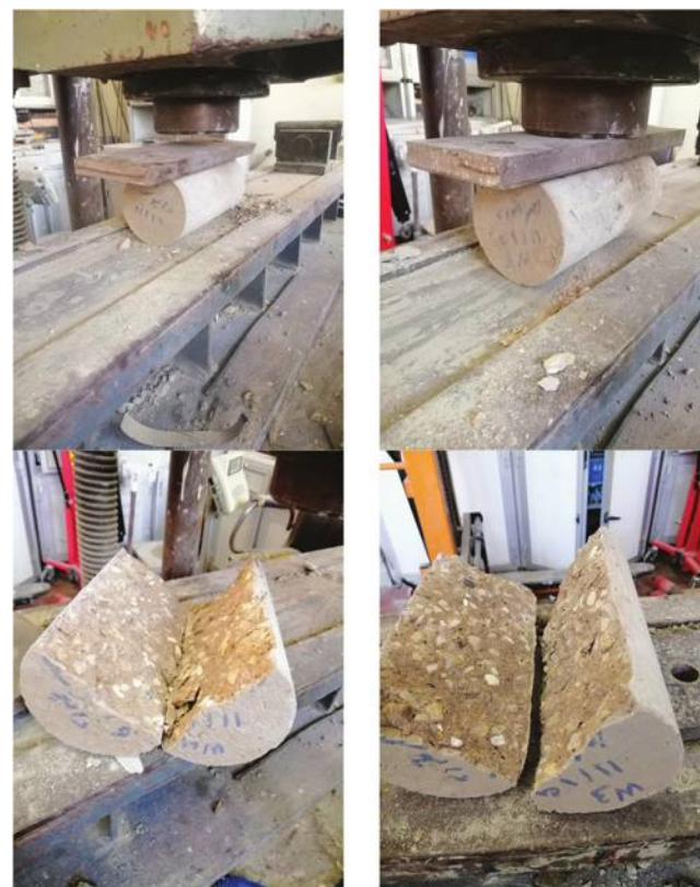
Fig. 11—Live photos during splitting strength measuring.
