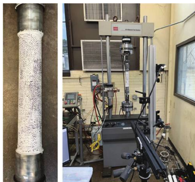
Fig. 5—Specimen speckle pattern and test setup with DIC system for Round 2.
