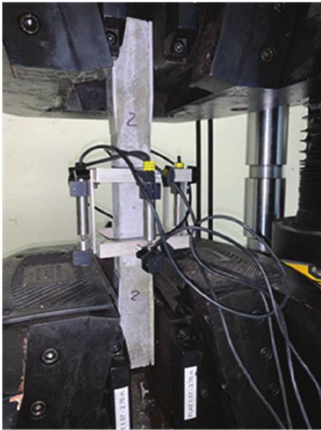
Fig. 1—FHWA direct tension test for UHPC.
