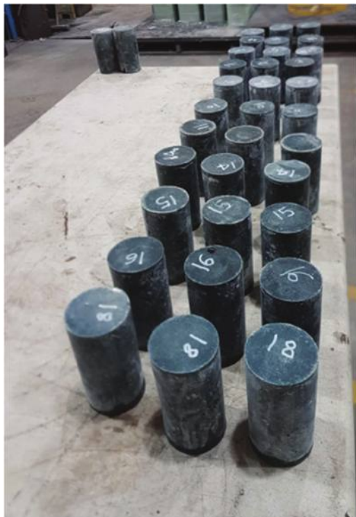
Fig. 1—AARPC specimens for compressive strength tests.
