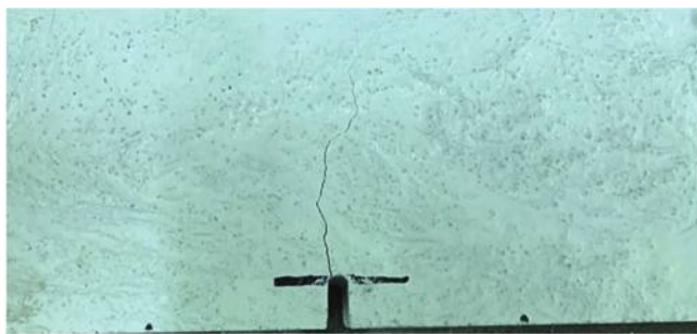
Fig. 9—Crack pattern in three-point bending in monolithically cast specimen.
