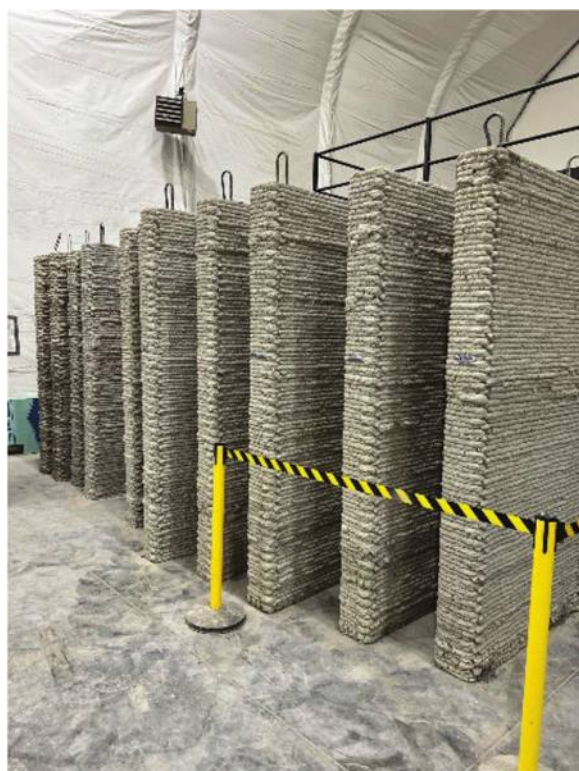
Fig. 17—8 ft (2.4 m) tall walls constructed in quasi-deployed conditions.
