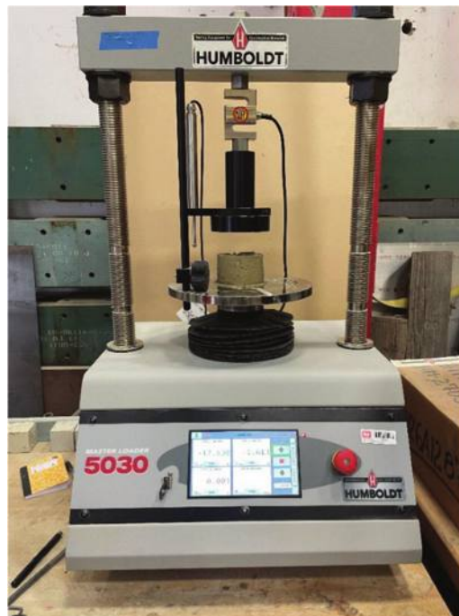
Fig. 4—Automatic unconfined compression test experimental setup.
