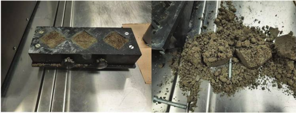
Fig. 7—Collapse of cube molds (setting time > 2 hours).
