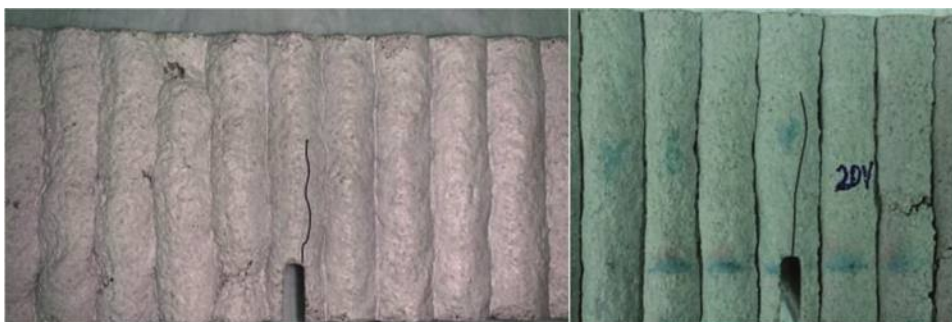
Fig. 11—Crack pattern in three-point bending in printed specimen with layer orientations parallel to loading.
