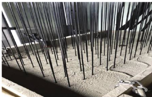
Fig. 11—Dry bed water and chemical injection and diffusion through 3-D printer's needle.
