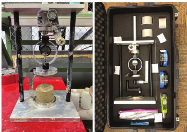
Fig. 3—Manual unconfined compression test experimental setup and storage in hard travel case.
