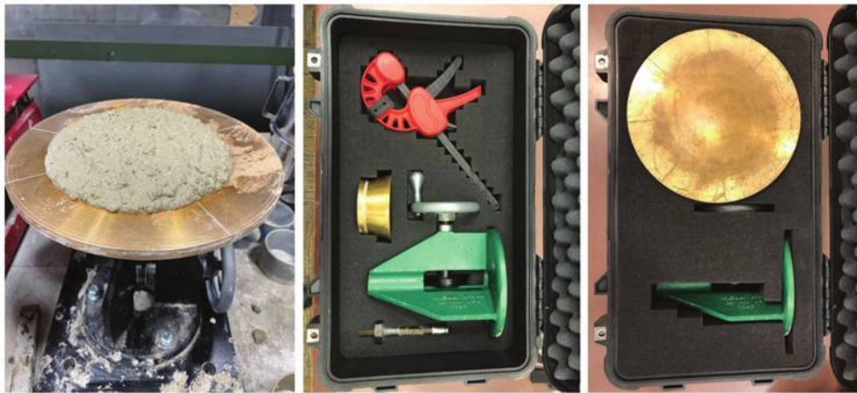
Fig. 2—Flow-table test experimental setup and storage in hard travel case.
