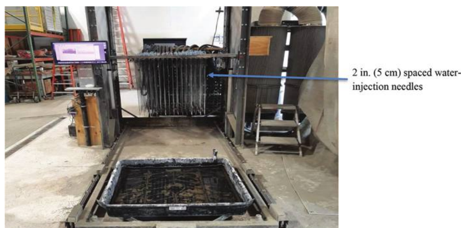
Fig. 2—Dry-bed technology for 3-D printing.
