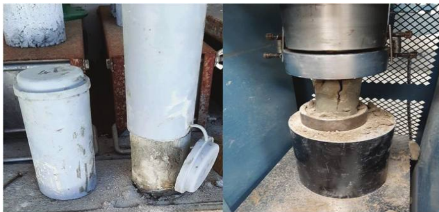
Fig. 9—Mold stripping and compressive strength testing.
