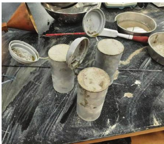
Fig. 8—Cylinder molds for mortar setting time evaluation.
