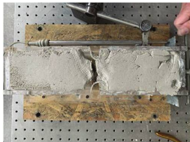
Fig. 3—Typical failure patterns in tensile and shear tests.
