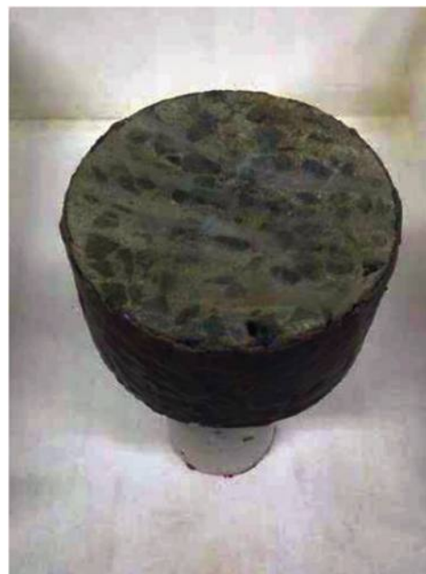
Fig. 7—Coating of specimens with epoxy.
