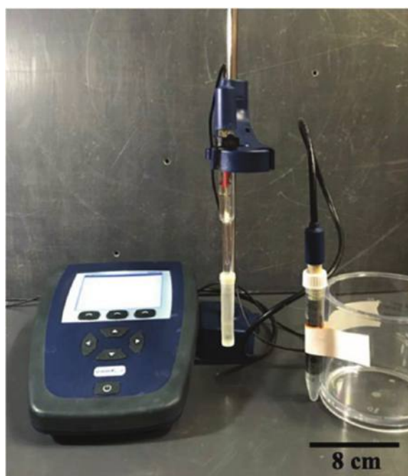
Fig. 2—Electrochemistry benchtop meter with pH probe (left); and resistivity probe testing specimen (right).
