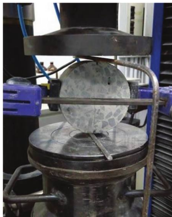
Fig. 6—Crack opening procedure.
