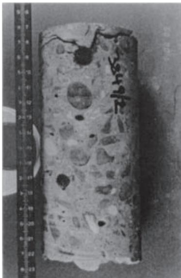
**Figure 6.9** Plastic settlement crack.
