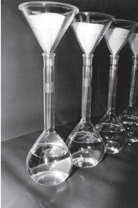
**Figure 4.2** Separation of silica from the concrete extracts.
