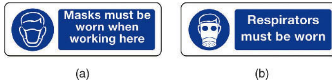
Figure 4.3 Breathing protection signs.
