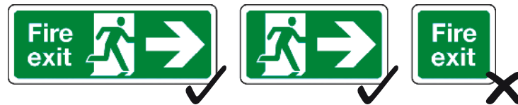
Figure 1.7 Text-only safety signs do not comply.
