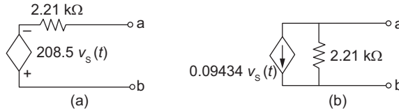
Fig. 5.6-2 (a) Thevenin's equivalent circuit for the amplifier in Example 5.6-1 (b) Norton's equivalent circuit
