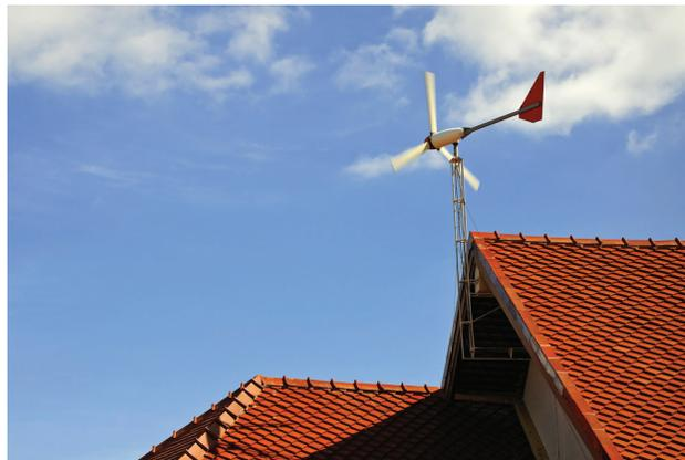
Figure 11.17 Mast mounted turbine.
