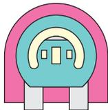
Figure 20.3 Preset resistor.
