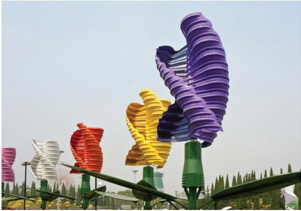
**Figure 11.18** Vertical axis turbine.
