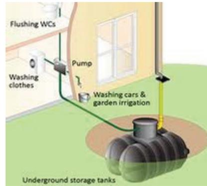
Figure 11.26 pumped system.
