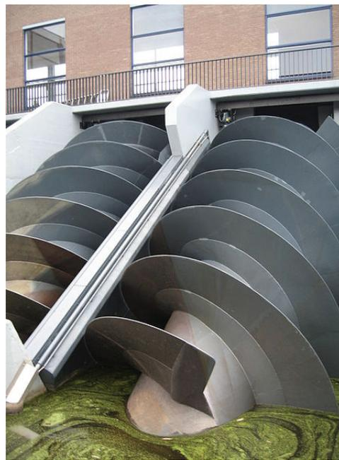
**Figure 11.20** The Reverse Archimedes Screw. Picture by M.A. Wijngaarden. Source: Wikimedia Commons.
