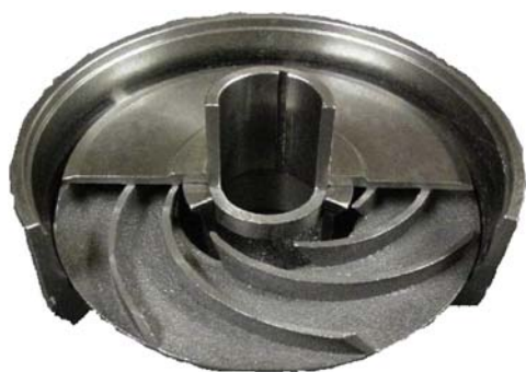
FIGURE 2.7 Impeller with top shroud partly removed.
