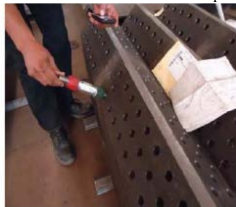
Figure 2 - An inspector checks bolt hole diameter (Photo courtesy Southern California Edison)
