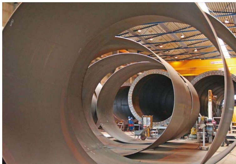
Photo 3 – Roll Formed Steel Sections - Courtesy Trinity Structural Towers
