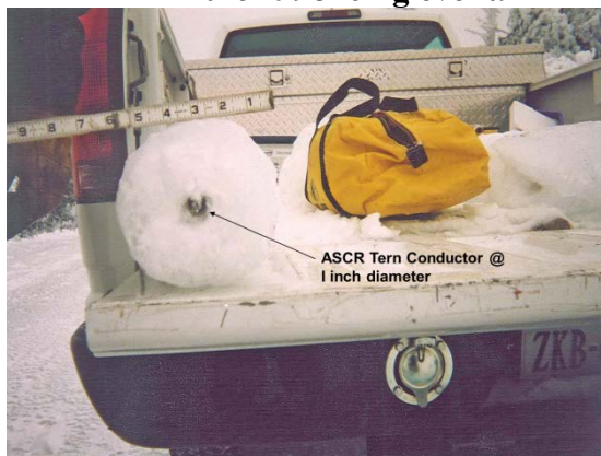
Figure 2 - Sample of 138kV conductor from the 1998 icing event.
