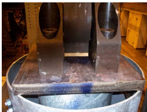
Figure 7. Close Up Photograph of Actuator to Inner Pipe for Prototype Test
