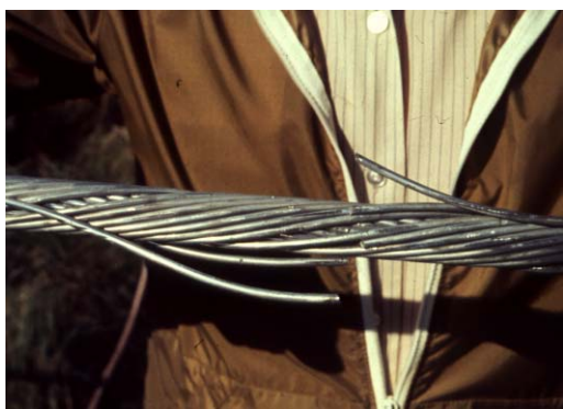
Figure 6a – Fatigue of Outer Strands
