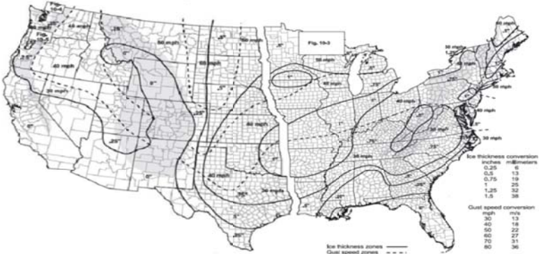
Figure 3 Extreme Ice and Concurrent Wind Map (ASCE 7-10); Figure 10-3 of ASCE 7 is also of interest for this paper (MRI = 50 Years)
