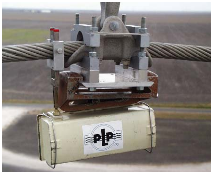
Figure 10 – Ontario Hydro Vibration Recorder
