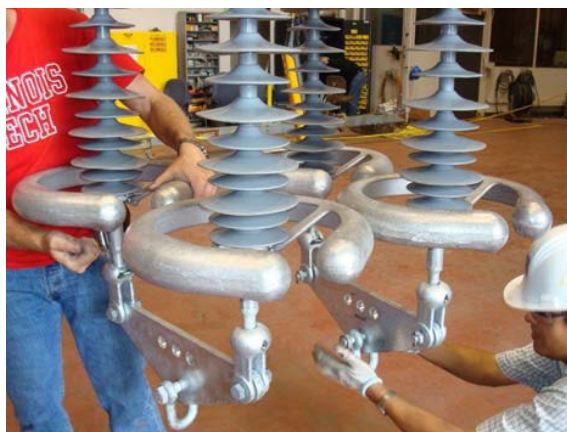
Figure 3 - Inspectors prepare insulators for corona testing (Photo courtesy Southern California Edison)
