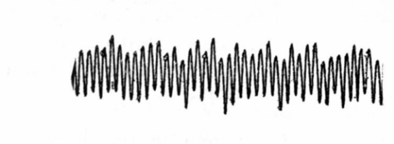
Figure 3 – 3/8” Overhead Shield Wire ( 41 Hertz)
