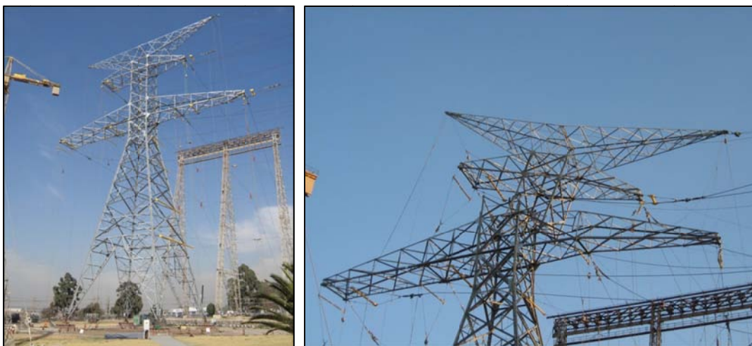
Figure 3. D5E NESC Heavy test, and top section failure, Johannesburg, SA.
