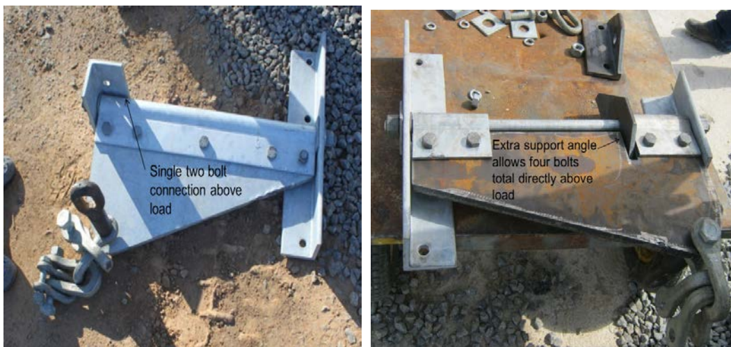
Figure 6 - Failed bracket configuration Figure 7 - Configuration passing testing
