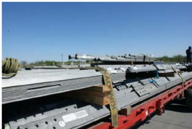
Figure 5 – Lattice Tower Steel ready for shipment (Photo courtesy Southern California Edison)
