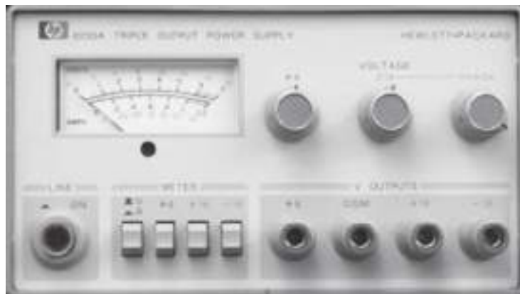
Figure 7.23 Example of a full-featured instrumentation power supply.
