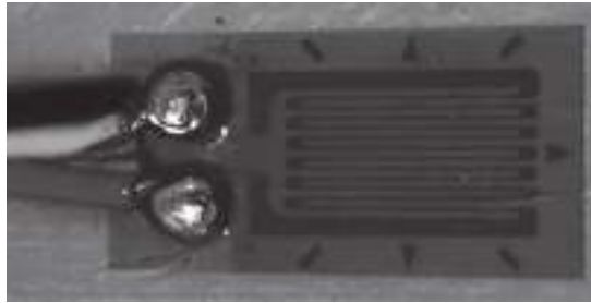
Figure 9.22 Mounted gage with three-wire connection. Courtesy of Measurements Group Inc., Raleigh, NC
