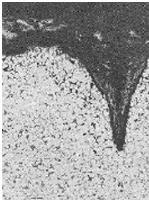
Figure 11.18 Corrosion fatigue crack. (From Source: NALCO Bulletin No. 70, NALCO Chemical Co.)
