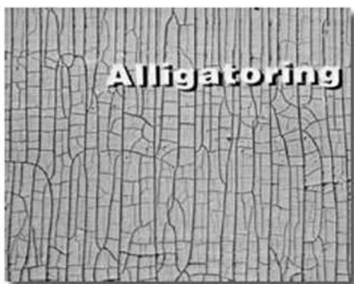
Figure 7.13 Alligatoring (Courtesy: Sigma Coatings)
