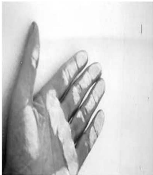
Figure 7.11 Chalking (Courtesy: Sigma Coatings)
