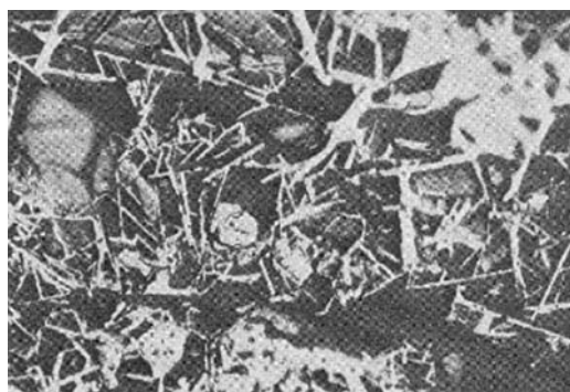
Figure 11.19 Caustic gouging of low-carbon steel. (From Wyncott, D. (1979). (NALCO), Corrosion in Boiler and Condensate Systems, Plant Eng. , October 18)
