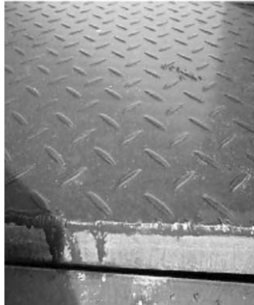
Figure 7.20 Holidays/Misses (Courtesy: Sigma Coatings)
