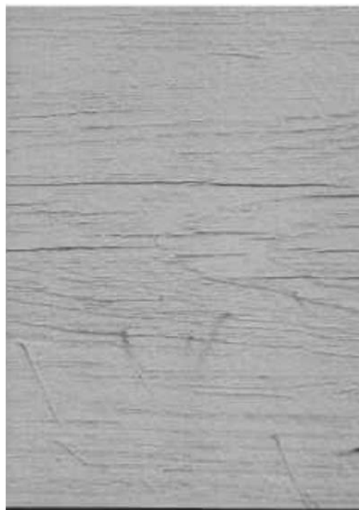
Figure 7.12 Checking (Courtesy: Sigma Coatings)
