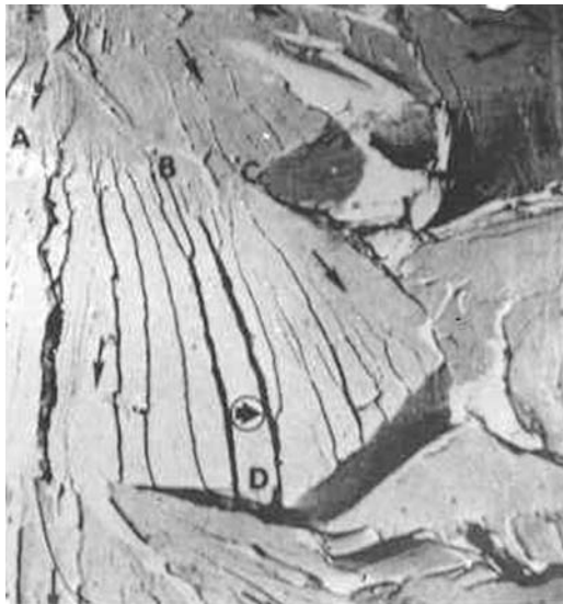
Figure 4.46 Typical cleavage fracture in iron
