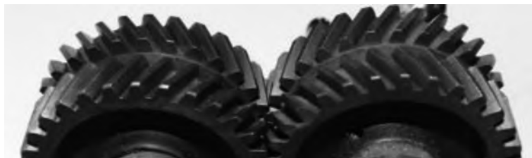
Figure 8.6 A herringbone gearset. (Courtesy of Matzner Photography, Madison, WI.)
