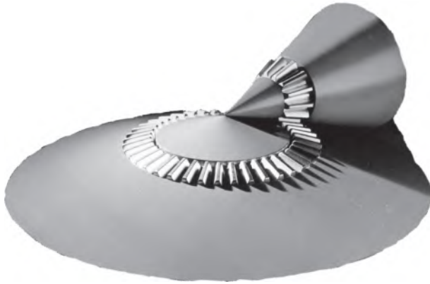
Figure 8.8 The pitch surfaces of bevel gears are cones that have only rolling contact. (Courtesy of Gleason Works, Rochester, NY.)
